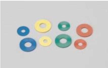
Color grease fitting washers are available in two sizes to fit 1/8 NPT or 1/4-28 grease fittings. Choose from red, blue, yellow, and green Buna-N washers to indicate grease type or relubrication frequency. Available in bags of 10 washers, all one color.
