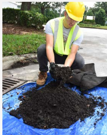
Actual contents of a 2-month Drain Guard test.
